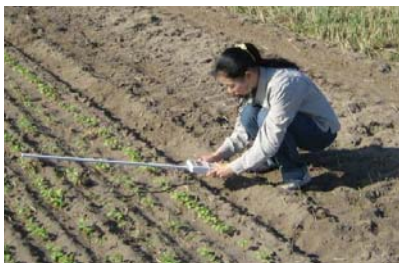
Pei-wen Huang measuring photosynthetic active radiation with an Accu-PAR LP-80 Ceptometer in 2 week-old buckwheat.
